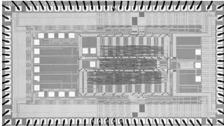
**Figure 3.** Microphotograph of the CMOS ASIC used as the processing element in this multiprocessor system. Eighty-six wire bonded pads are shown at the chip perimeter. Other unbonded pads are for probe-testing
