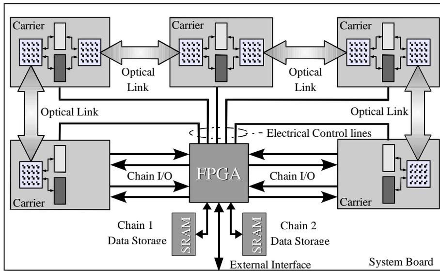
**Figure 1.** System diagram showing five carrier boards placed on system board. OptoElectronic arrays are shown on left and right sides of carrier boards and processing elements in the center of the carrier boards. The upper (*light*) PEs indicate one chain and the lower (*dark*) PEs indicate the second chain
