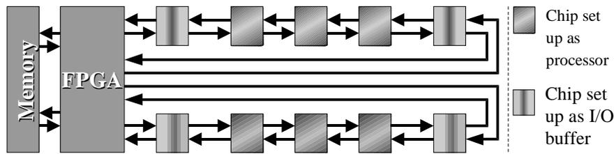
**Figure 2.** Diagram of logical connection between the multiple processors and the FPGA controller and memory. The upper and lower chains here illustrate the two independent chains in this system
