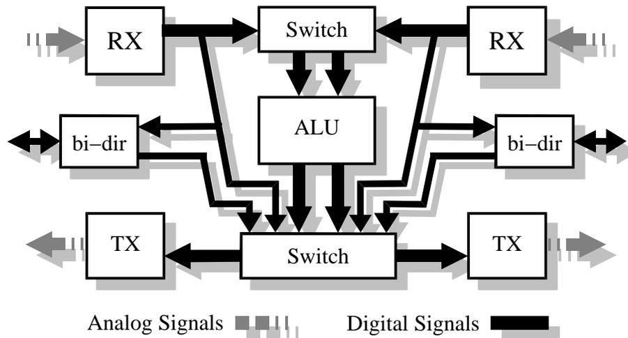
**Figure 4.** Architecture diagram of the processor element showing dataflow through the chip. (*Thinner*) lines indicate dataflow pattern when by-passing the computational portion of the chip
