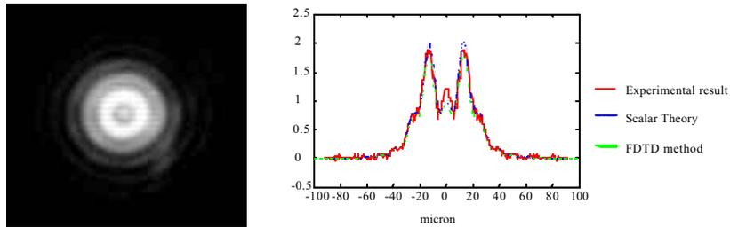
**Fig. 8.** Comparison between experimental results and theoretical predictions for the diffraction from a precision pin-hole that had a diameter of 71 microns at an axial location of 350 microns.
