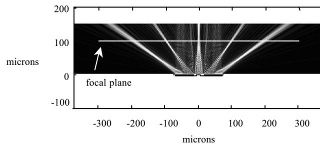
**Fig. 3.** Illustration of a VLSI-scale 1-to-5 fan-out DOE, computed using the boundary element method. The width of the DOE is 120 microns and the focal length is 100 microns.
