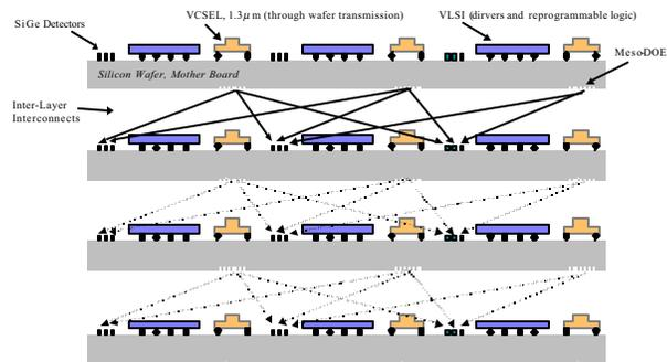
**Fig. 1.** Monolithic interconnect architecture that uses 3D diffractive optical interconnects on the VLSI-scale for through wafer fan-out interconnects for data or clock distribution. Various modules of this architecture can also be stacked together to realize more complex systems.
