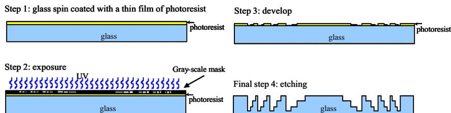
**Fig. 4.** Graphical illustration of the gray-scale photolithographic fabrication process.
