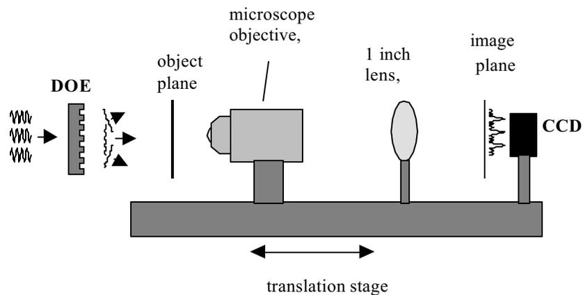
**Fig. 7.** Micro 4f imaging system for characterizing mesoscopic diffractive optical elements.
