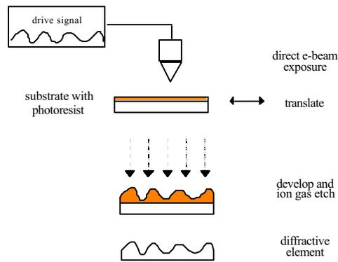
**Fig. 5.** Fabrication process for continuous profile DOEs based on direct electron beam write.
