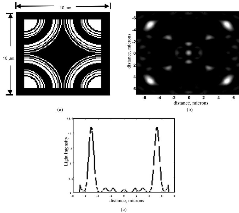
**Fig. 2.** Illustration of a three dimensional subwavelength off-axis lenslet array used for 1-to-4 fanout on the VLSI-scale (a) DOE, (b) intensity image in the focal plane, and (c) line scan thorough the focal plane. Results were generated using a 3D FDTD diffraction model.
