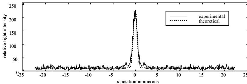
**Fig. 9.** Overlay of the experimental characterization of a mesoscopic diffractive lens and the results predicted from our electromagnetic models. Data was taken from our system using a 40X magnification objective at the location of  $z=65\mu\text{m}$ , the design focal length.
