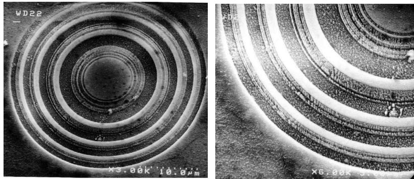
**Fig. 6.** Illustration of a mesoscopic diffractive lens having a diameter of 36 $\mu\text{m}$ , a focal length of 65 $\mu\text{m}$  and a minimum feature size of 60nm. The element was fabricated by Dr. Axel Scherer, of the California Institute of Technology.
