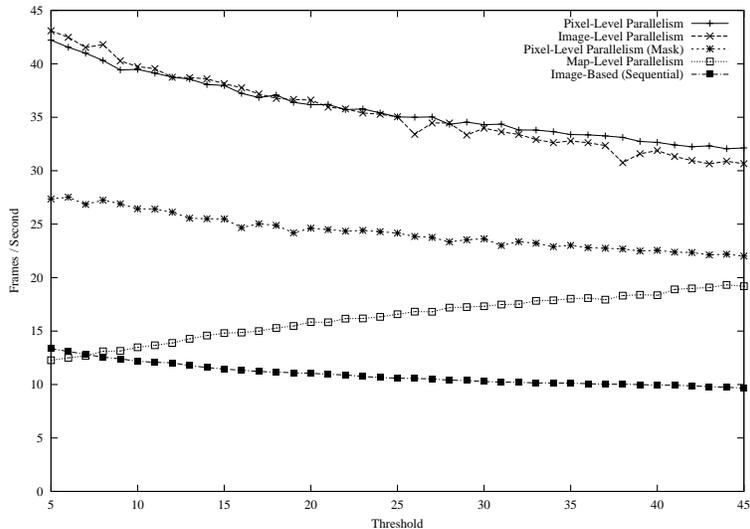
**Fig. 5.** System throughput of algorithms on multiprocessor architecture.
