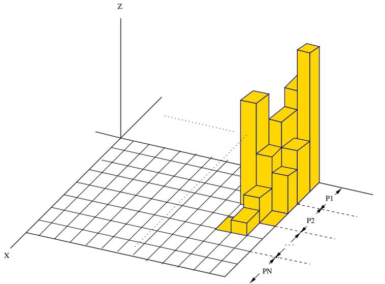
Fig. 4. The processor workload using map-level parallelism.
