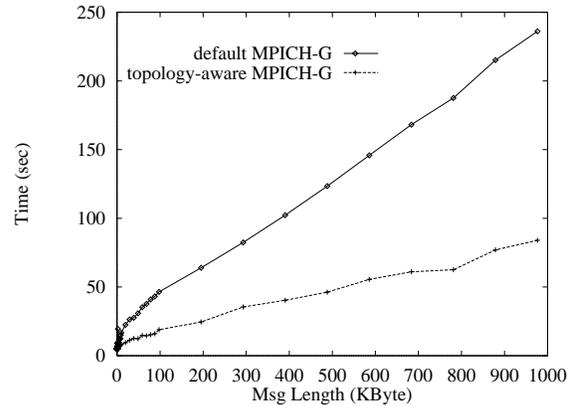
**Figure 7. Original MPICH broadcast vs. topology-aware MPICH broadcast across a wide-area network running 16 processes on the IBM SP at SDSC, 16 processes on the IBM SP at ANL, and 16 processes on the SGI Origin2000 at ANL.**
