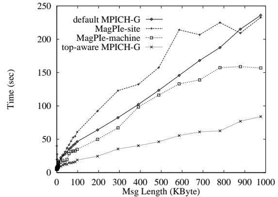
**Figure 9. Original MPICH broadcast vs. topology-aware MPICH broadcast vs. MagPIe broadcast across local- and wide-area networks running 16 processes on the IBM SP at SDSC and 16 processes on each the IBM SP and SGI Origin2000 at ANL.**
