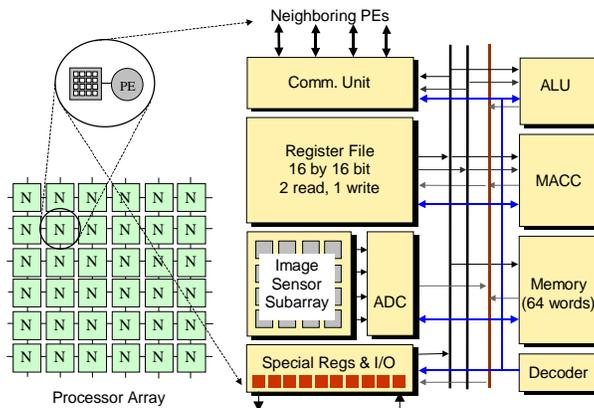
**Fig. 1.** Block diagram of the SIMPil SIMD system
