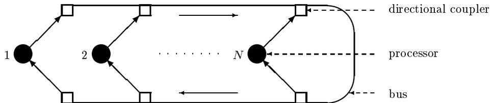
**Fig. 2.** Fiber optic bus with directional couplers.
