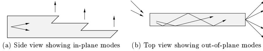
**Fig. 4.** In-plane and out-of-plane modes of a slab waveguide; for simplicity only a portion of the slab is shown.
