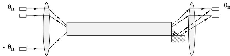
**Fig. 7.** Multiple out-of-plane modes entering and exiting a slab. The figure shows a top view of the slab. For clarity, only light entering from one input port and leaving through a one exit port of the slab have been shown.
