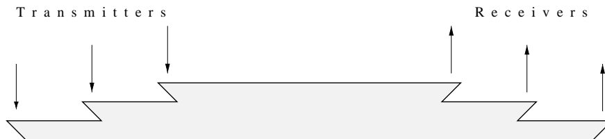
Fig. 3. The sawtooth slab waveguide; in this figure, the plane of the slab is the plane of this page; a view of this plane will be called the side view . The direction perpendicular to the plane of the slab will be termed the top view .
