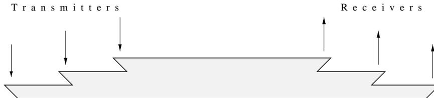
**Fig. 3.** The sawtooth slab waveguide; in this figure, the *plane of the slab* is the plane of this page; a view of this plane will be called the *side view*. The direction perpendicular to the plane of the slab will be termed the *top view*.
