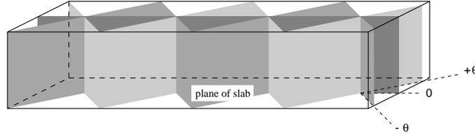
**Fig. 5.** A section of the slab, showing three out-of-plane modes. These modes are well separated as they propagate in different angles when viewed in a direction perpendicular to the plane of the slab (top view). In the plane of the slab itself, the modes are well mixed.
