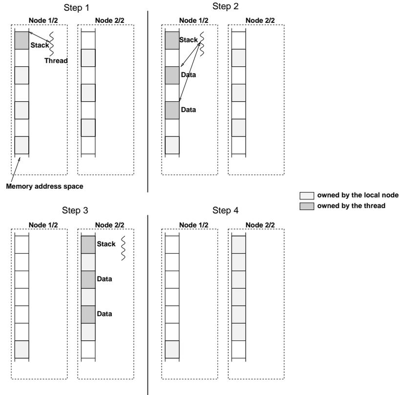
**Fig. 6.** Slot ownership may change due to migration. In this example, a thread is created and acquires a slot owned by the local node to store its stack (Step 1). The thread acquires other slots from the local node, to store its private data (Step 2). The thread migrates along with its slots (Step 3). The thread dies and its slots are acquired by the destination node (Step 4).
