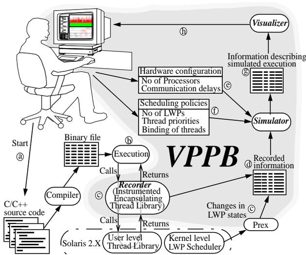
**Figure 1: A schematic flowchart of the VPPB system.**
