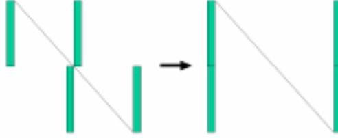
**Fig. 6.** N-Merge algorithm for banded linear systems merges two N-shaped non-zero bands of height  $m$  to one N-shape of height  $2m$ , and thus eliminates all the non-diagonal elements in  $\log(n)$  parallel steps for a system of size  $n$ .
