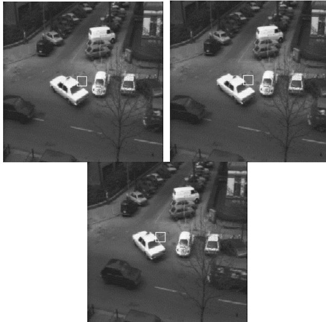
Fig. 3. Three frames of a test image sequence, in which a taxi is seen turning a corner at an intersection. The target to be tracked was taken from the center of the first frame (not shown). White rectangles of size 16 \times 16 represent the best matches found in each image, relative to the target's appearance in the previous image.
