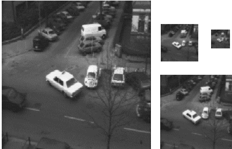
Fig. 2. Four levels of a Gaussian pyramid. These were computed by Splash 2 from a 512 \times 512 image which is not shown. The image sizes here are 256 \times 256 , 128 \times 128 , 64 \times 64 , and finally 32 \times 32 , which serves as the coarsest level in this implementation.
